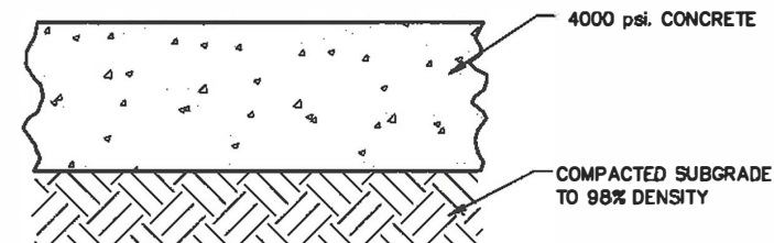
B4 SECTION - TYPICAL 6 INCH CONCRETE PAVEMENT C-116 SCALE: NTS
